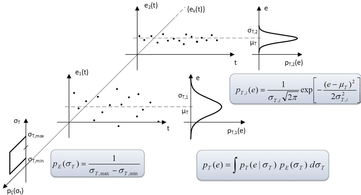
Figure 7: PES modelled as time- and ensemble-random variable (t, k)
