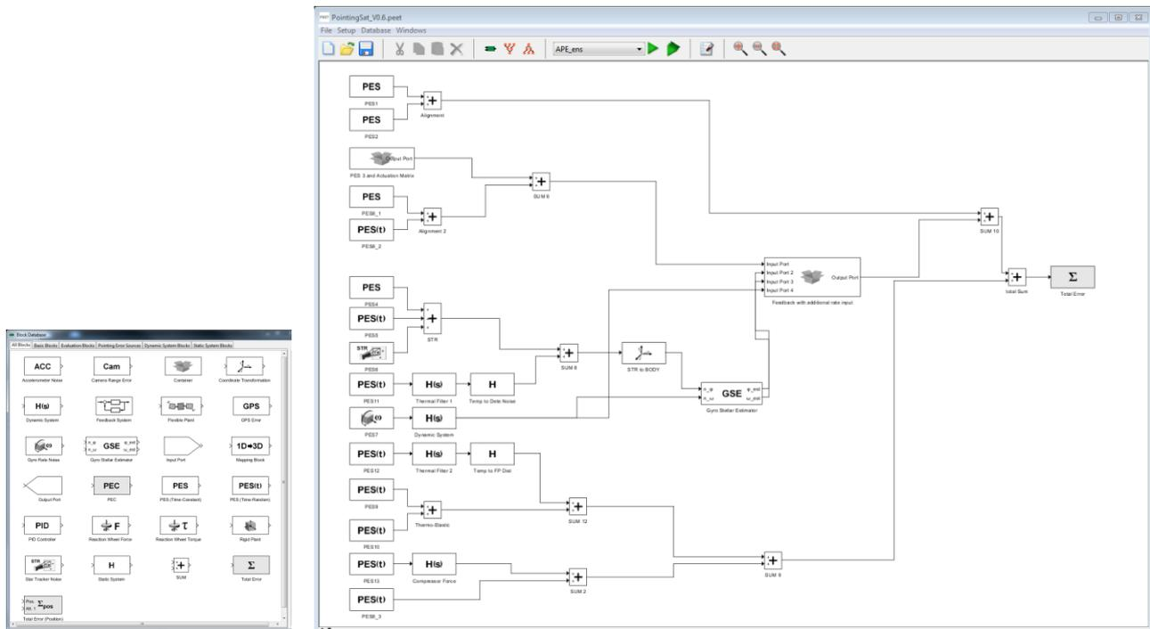
Figure 12: PEET v1.0 block database (left) and system editor (right)
