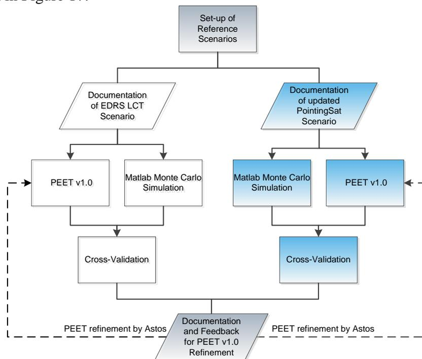
Figure 17: Cross-validation process for PEET v1.0
