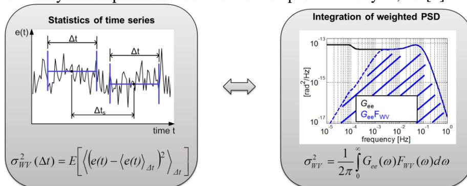
Figure 5: Exact correspondence of the time-windowed statistics of a time-series and the integration of a corresponding weighted PSD
