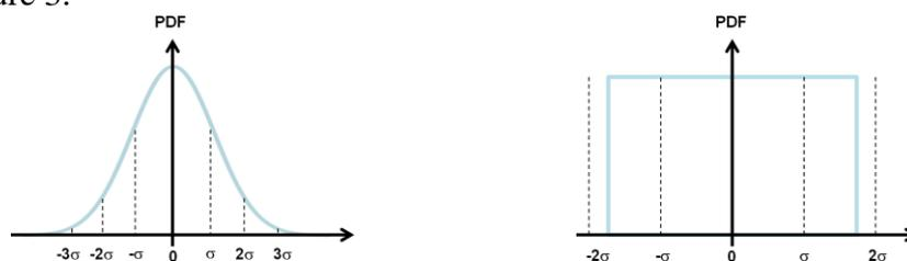
Figure 3: Error evaluation with confidence coefficients - correct results for a Gaussian distribution (left) and significant deviation for non-Gaussian distribution (right)
