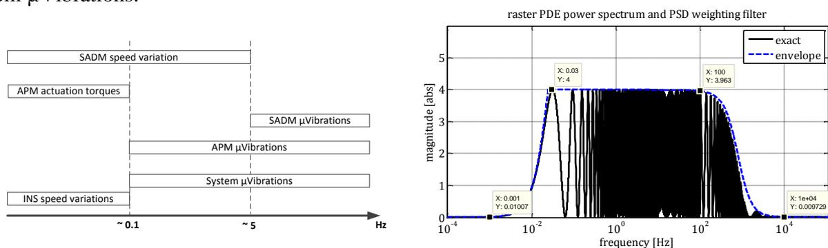
Figure 21: Interdisciplinary MetOp-SG PES in the frequency domain (left) and the corresponding frequency domain metric for evaluation (right), cf. [1].
