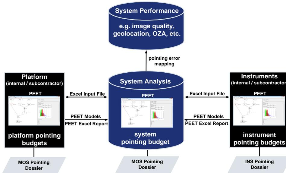
Figure 18: MetOp-SG pointing error engineering process
