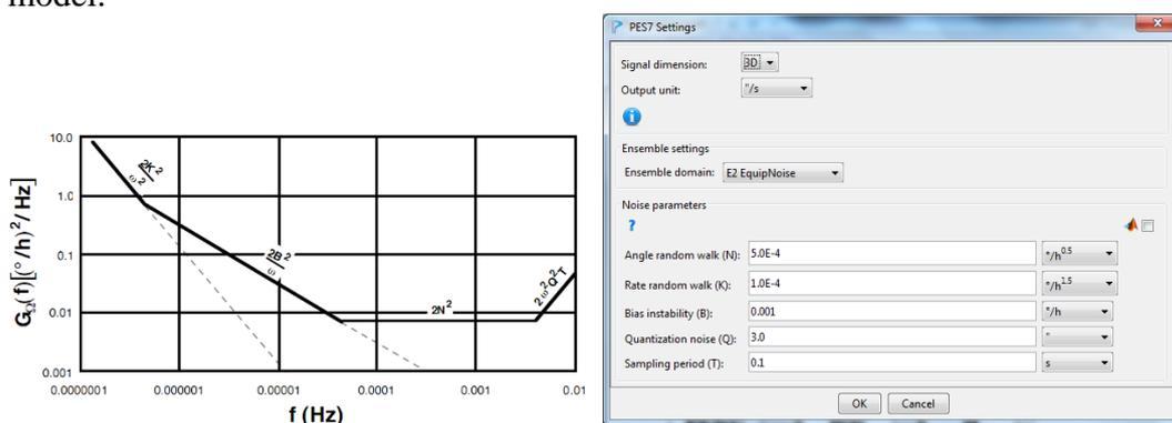
Figure 13: Gyro IEEE model (left) and the corresponding interface of the model block in PEET v1.0 (right)
