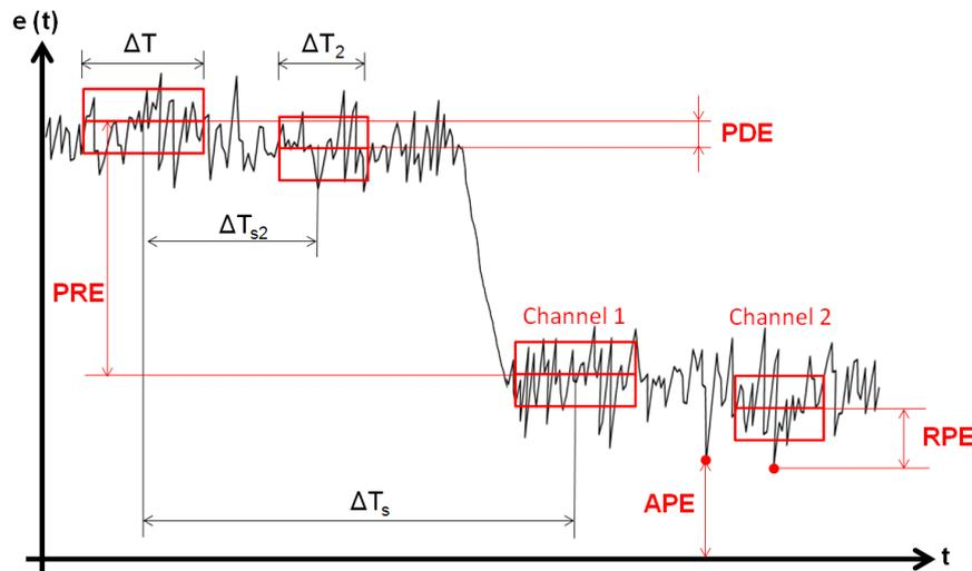
Figure 9: PointingSat Error Indices
