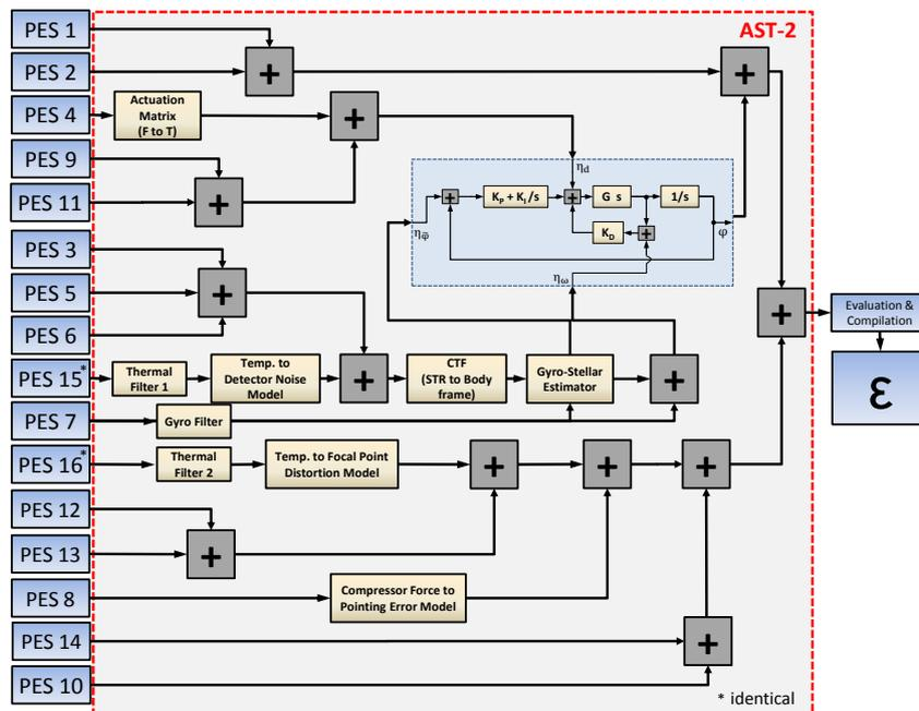
Figure 11: PointingSat schematic break-down in PES, system transfers and summations
