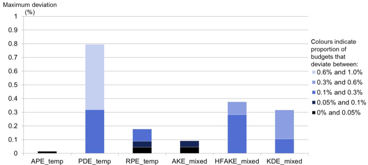
Figure 20: Deviation of results obtained with PEET v1.0 and PEET v0.6 for the MetOp-SG platform pointing budgets
