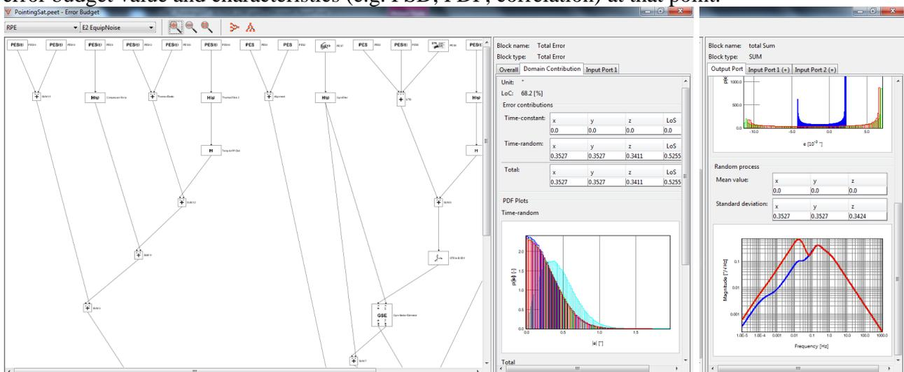
Figure 15: Tree-view of the PointingSat pointing error budget with PDF (left) and PSD (right) characteristics.
