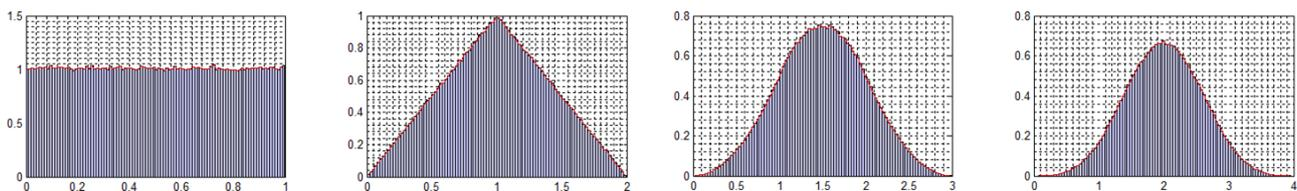
Figure 2: Simplified Statistical Method - Example: Sum of uniform distributions converge to Gaussian distribution
