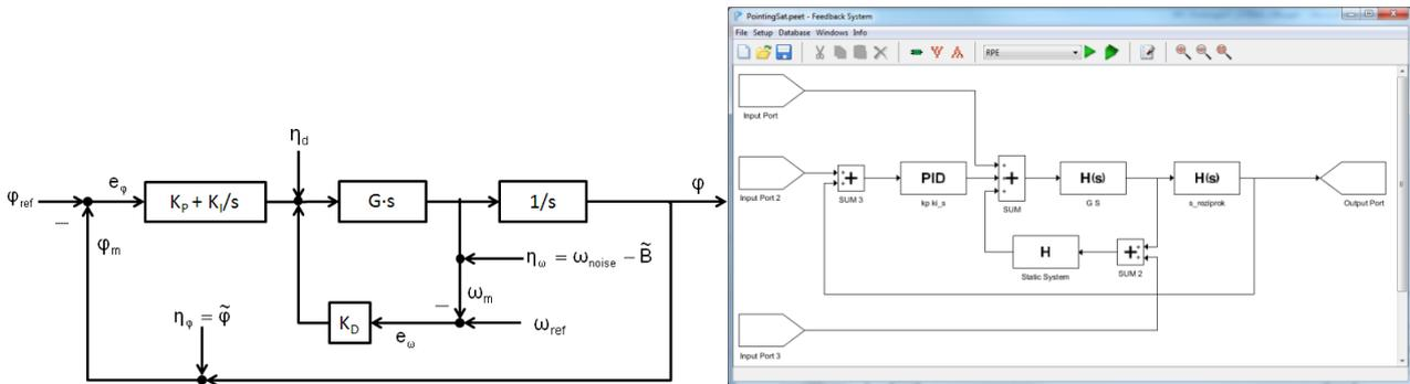
Figure 14: Schematic closed-loop control transfer (left) and the corresponding closed-loop editor in PEET v1.0 (right)
